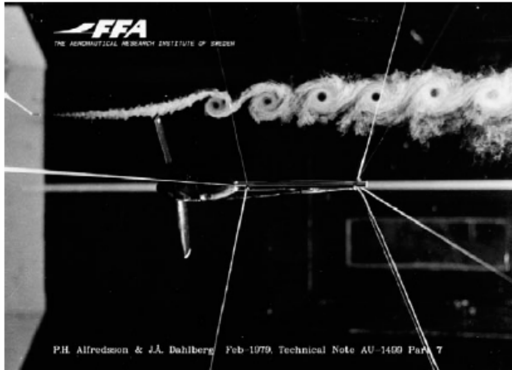
Fig. 4. Flow visualisation with smoke, revealing the tip vortices (from [16]).
